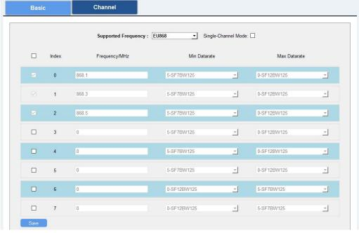
If frequency is one of CN470/AU915/US915, you can enter the index of the channel that you want to enable in the input box, making them separated by commas.
