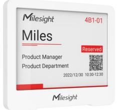
DS3604 is a reflective electrophoretic display offering readability and flexibility. The 4.2-inch active area contains 400 x 300 pixels and has 1-bit Black/White/Red full display capabilities. DS3604 supports displaying up to 150 languages and other modules like picture or QR code. Long-capacity batteries and ultra-low power consumption bring a long battery life of up to 5 years.
