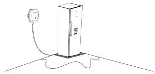
To ensure the most sensitive effect, ensure the installation location is a flat surface without debris, dust and deep gaps. If the membrane needs to be pasted to installation location, the surfaces should be cleaned and free from dirt, adhesive residue, water drops and other things.
