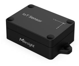
EM310-TILT is a LoRaWAN® tilt sensor mainly for angle measurement and asset movement detection. With a compact size and 3-axis accelerometer, EM310-TILT can be installed to the objects easily to measure its X, Y, Z tilt angles. It can also detect the movement based on angle changes and send threshold alarms. Compliant with Milesight LoRaWAN® gateway and Milesight IoT Cloud solution, users can know the angles and tilt threshold alarms in real-time via browser or mobile app remotely.
