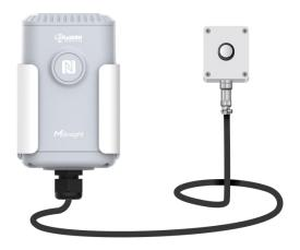
EM500-LGT is designed for measuring light in harsh environments and transmitting data using LoRaWAN® technology. With this low power consumption technology, EM500-LGT can work up to 10 years with 19000 mAh battery. Combining with Milesight LoRaWAN® gateway and Milesight IoT Cloud solution, users can manage all sensor data remotely and visually.
