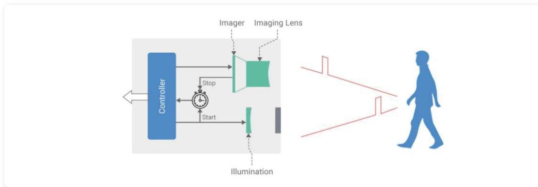
**iToF:** The full name is Indirect Time-of-Flight, indirectly measures the flight time of light by the phase difference. The iToF module emits a modulated infrared signal into the scene, then receives the light signal reflected from the object detected, and calculates the phase difference between the emitted signal and the received signal according to the accumulated charge during the exposure time. It will get the depth information of the target object via the processes.
