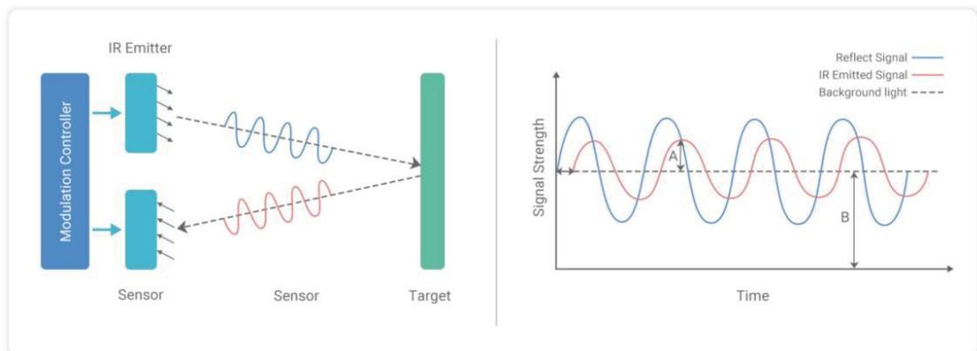
The ToF technology consists of dToF (direct Time of Flight) and iToF (indirect Time of Flight) which are distinguished by different detection methods.
