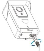
**Step 8:** Connect the device to the backplane that you've installed already and tighten the fixing screws. Then the installation is completed.
