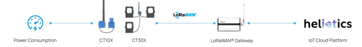
With the help of Heliotics, the customer successfully deployed a non-intrusive power monitoring solution featuring Milesight CT10x Smart Current Transformers to provide real-time energy insights without disrupting operations. This IoT-based system enables remote monitoring, predictive maintenance and data-driven decision-making, helping to optimize efficiency and reduce costs. Around 30 devices were deployed across 10 machines and the CT10x was deployed on almost every machine in the factory.
