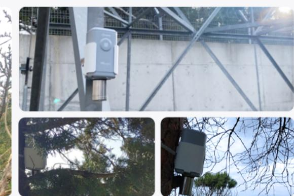
For Forest Fire Prevention, installed on radio towers throughout the city, the Milesight EM500-CO<sub>2</sub> sensors can provide accurate environmental data by continuously monitoring temperature and humidity in real time, detecting the critical parameters that indicates the happening of fire.
