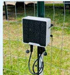
The UC511 connects directly to a DC latching solenoid to control the valve's open/ close status. It receives wireless commands over LoRaWAN® based on environmental data collected by third-party sensors, such as soil moisture, temperature, and humidity. This enables precise, automated irrigation aligned with real-time field conditions.
