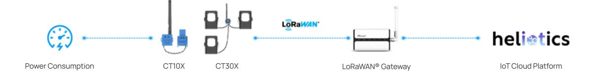
With the help of Heliotics, the customer successfully deployed a non-intrusive power monitoring solution featuring Milesight CT10x Smart Current Transformers to provide real-time energy insights without disrupting operations. This IoT-based system enables remote monitoring, predictive maintenance and data-driven decision-making, helping to optimize efficiency and reduce costs. Around 30 devices were deployed across 10 machines and the CT10x was deployed on almost every machine in the factory.
