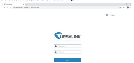
If the SIM card is connected to cellular network with public IP address, you can access WEB GUI remotely via the public IP address when remote access is enabled.
