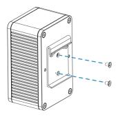
2. Hang the device to the DIN rail. The width of DIN rail is 3.5cm.
