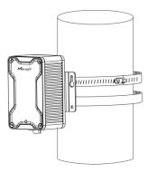
**Note:** UPS and the terminal device can be fixed together with the same hose clamp. When being installed together, the UPS can be wrapped by only one hose clamp.
