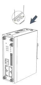
B. Put SIM card onto the slot then insert the back into the hole.
