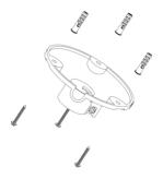
**Step 8:** Fix the pole to bracket base with L-shaped screwdriver.
