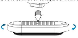
**Step 3:** Gently rotate the black knob in the direction shown to loosen it, then adjust the direction of 3-axis ball.
