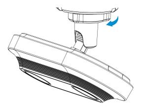
Step 4: After the installation angle is set, tighten the knob in the direction shown to secure the device.
