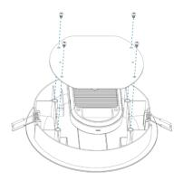
Step 3: Adjust spring buckle to vertical state, then mount the cover to the ceiling.
