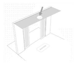
**Step 2:** Place the device into the cover, then fix the cover plate to the cover via screws.
