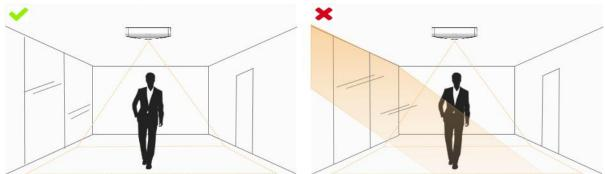
• Make sure there are no moving objects interfering in the counting area. For example, do not install the sensor too close to a door.
