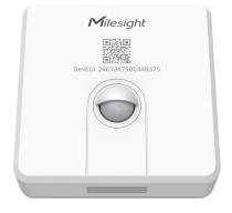
The Milesight WS203 is an environmental monitoring device that combines motion and temperature/humidity (TH) sensors. By detecting motion within an 8-meter range based on passive infrared (PIR) technology, the WS203 can trigger TH detection and periodically report environmental status over LoRaWAN® network.
