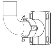
2. Connect one side of sensor cable to WTS Sensor and tighten the cable, pass the cable through the bent pipe and bracket, then connect the pipe to the bottom of sensor and fix both parts with 3 hex socket cap mounting screws.
