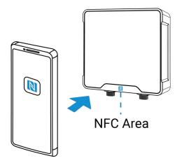
4. Basic information and settings of WTS Hub will be shown on ToolBox if it's recognized successfully. You can read and configure the device by tapping the buttons on the App. In order to protect the security of devices, password validation is required when configuring via unused phone. Default password is **123456**.
