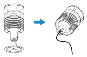
2. Connect the sensor to the pole top flange with nuts and bolts, then connect the other side of sensor cable of the right interface of WTS Hub. When installing, ensure the arrow on the sensor facing north according to a compass. Users can install the sensor with other installation methods by selecting other accessories.
