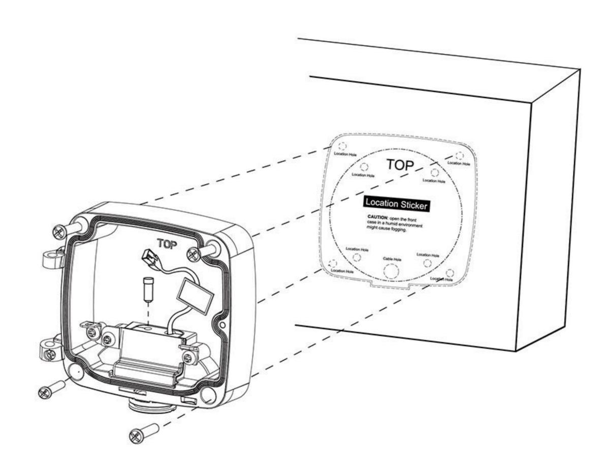
Step3: Remove tension disc and put the cables through the rubber plug. Afterwards, fix the tension disc again and then connect the cables correctly. After finishing the above steps, connect the camera body with the front cover.
