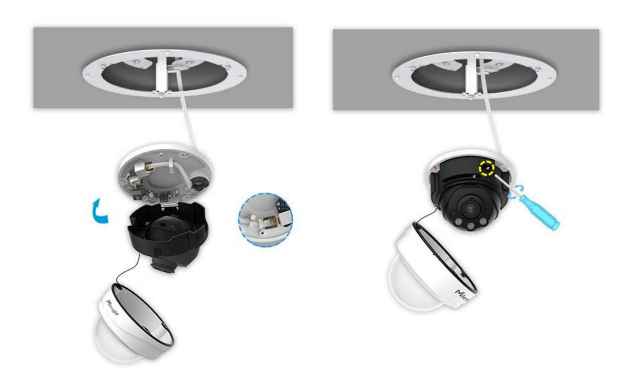
Step 12: Attach the dome cover by tightening 3 loosened screws on Step 3 and make sure that the groove on the dome cover is aligned to the one on the camera;
