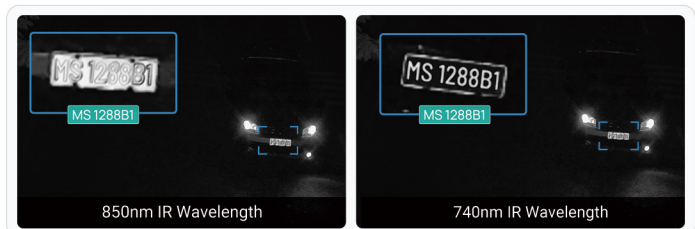
740nm/850nm Dual IR Wavelength
