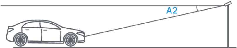
Figure 1-4 Installation Vertical Pitch Angle
