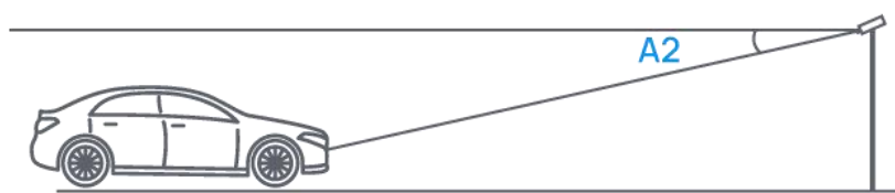
Figure 2-5 Installation Vertical Pitch Angle
