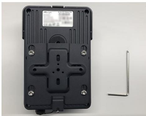
2. Use the screwdriver to remove the screws located at the bottom of the camera back panel, as shown in the diagram. The back panel can then be freely removed.
