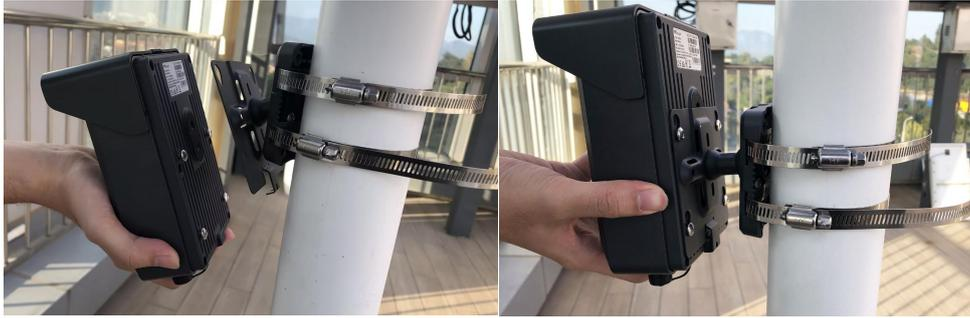
5. Reattach the previously removed screws to ensure the camera is secure and firmly fixed.
