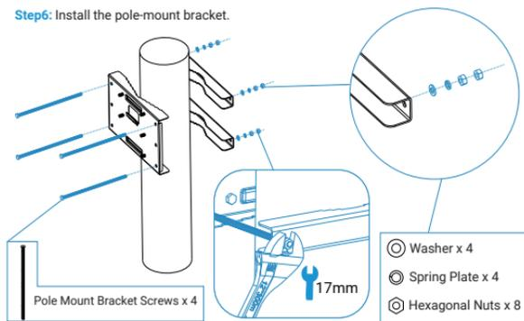
**Note:** The recommended diameter for the support columns is 150mm to 210mm.
