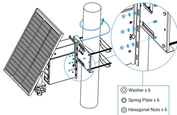
**Step9:** Secure the bracket using hex nuts.
