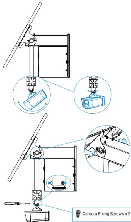
**Note:** You can also use expansion screws to mount the entire assembled bracket directly onto the wall.
