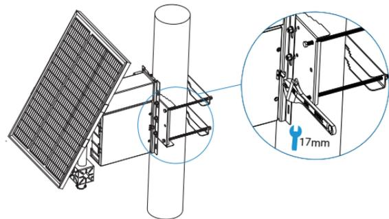
**Step10:** Use a safety latch to securely attach the camera to the bracket interface. Opening the front cover of the bracket allows for easier threading of the camera's tail cable through the interface to the battery system.
