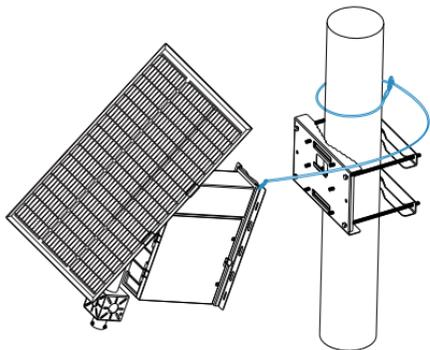
**Step8:** Hook the bracket onto the mounting hook on the pole.
