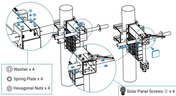
**Step2:** Secure the assembled solar panel to the additional bracket.
