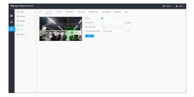
Auto Home allows the PTZ camera to return to a predefined Home Position automatically after a period of latency time. Check the checkbox to enable the Auto Home mode.
