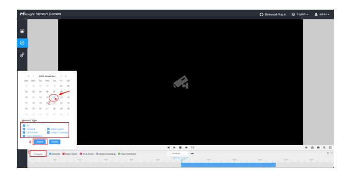
**Step2:** The timeline displays the video files for the day and show different colors according to selected record type. Drag the progress bar with the mouse to locate the exact playback point as needed.
