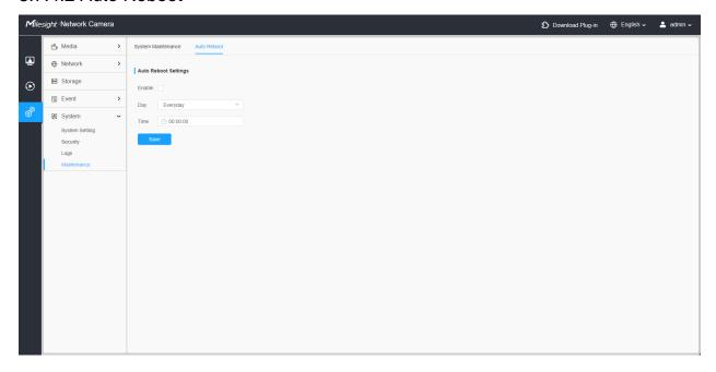
Set the date and time to enable Auto Reboot function, the camera will reboot automatically according to the customized time in case that camera overload after running a long time.
