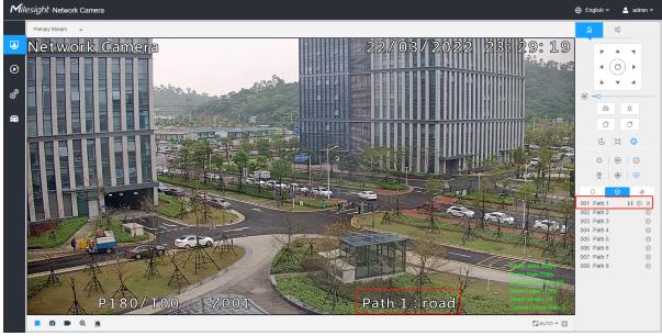
Step2: Use the PTZ control buttons to move the lens to the interested position;
