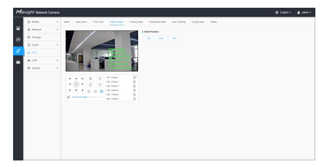
You can configure the Initial Position for PTZ cameras as a zero point.
