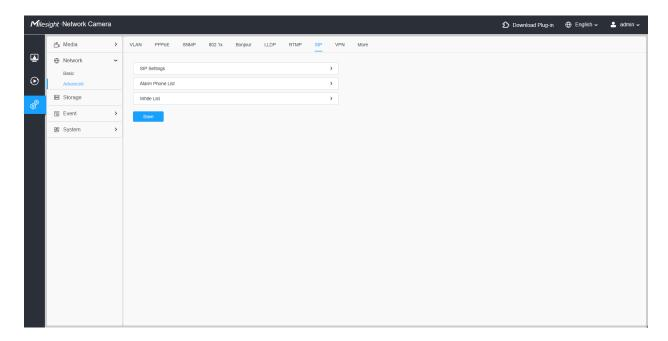
To use this function, the settings in SIP page must be configured properly. There are two ways to get video through SIP, one is to dial the IP address directly, the other is account registration mode. the details are as follows:
