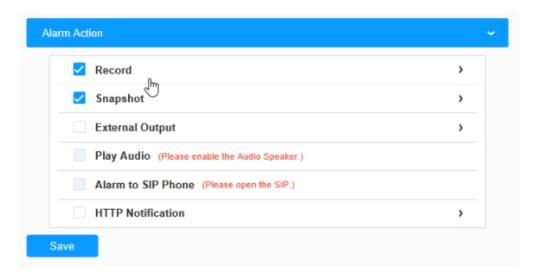
Click Save button to finished the configuration. The alarm will be triggered when workers in the detection area do not properly wear the hard hat, and an alarm icon will appear and the detection box will turn red.
