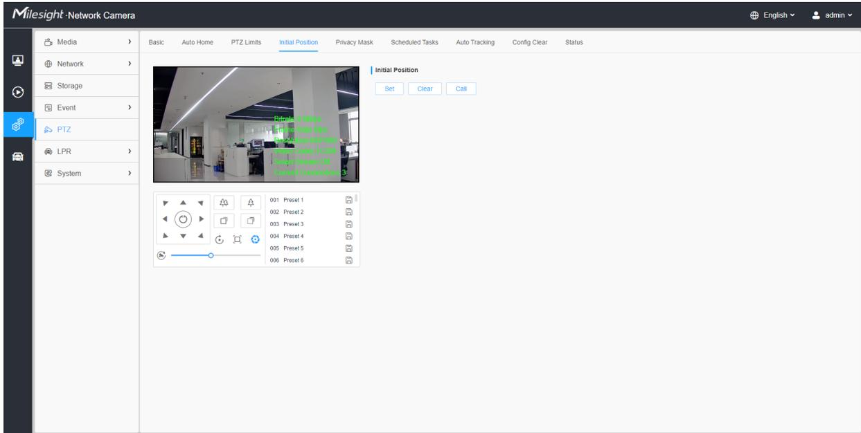
You can configure the Initial Position for PTZ cameras as a zero point.
