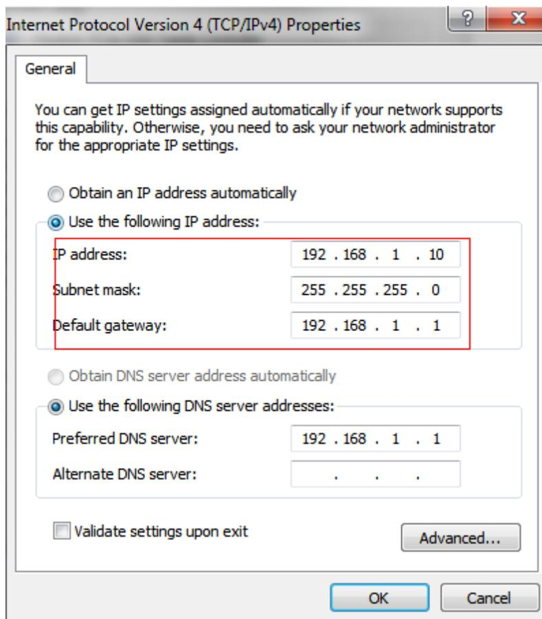
**b.** Click “Advanced”, and then click “IP settings”--> “IP address”--> “Add”. In the pop-up window, enter an IP address that in the same segment with Milesight network camera ( e.g. 192.168.5.61, but please note that this IP address shall not conflict with the IP address on the existing network);
