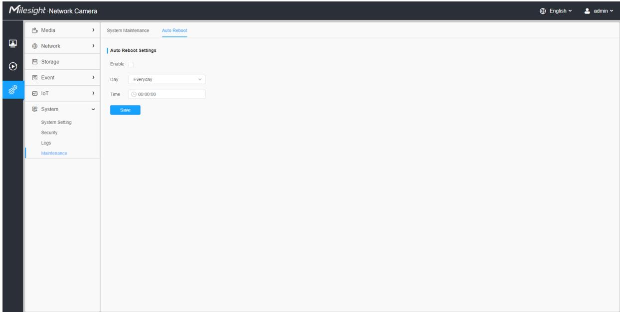
Set the date and time to enable Auto Reboot function, the camera will reboot automatically according to the customized time in case that camera overload after running a long time.
