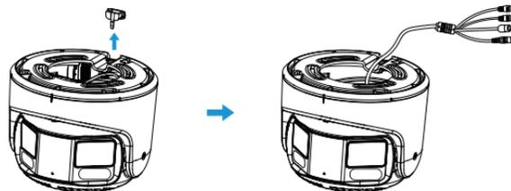
**Step4:** Install the camera to the mounting bracket by rotating it, ensure the installation marking is located between the two endpoints of the bracket mounting, and then tighten the horizontal limit screws.
