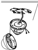
**Step3:** Rotate the camera unit clockwise, and then fix the camera to the bracket with the setscrew;
