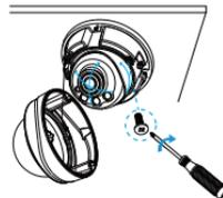
**Step6:** Attach the dome cover and make sure that the groove above is aligned to the one below as the picture shows, then fix the camera tightly.
